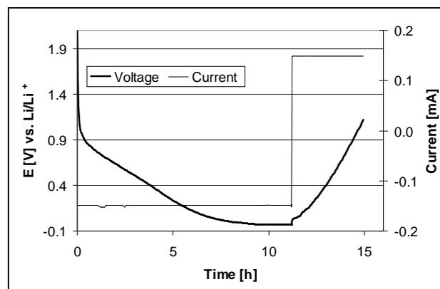
**Figure 1:** First galvanostatic lithium insertion into a phenolic resin-based carbon material (charge rate C/5, between 1.5 V and -30 mV vs. Li/Li<sup>+</sup>). The lithium insertion step was stopped during lithium plating.
