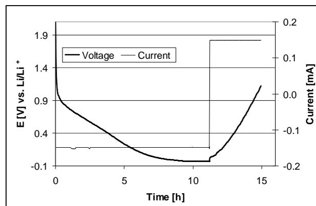
**Figure 1:** First galvanostatic lithium insertion into a phenolic resin-based carbon material (charge rate C/5, between 1.5 V and -30 mV vs. Li/Li<sup>+</sup>). The lithium insertion step was stopped during lithium plating.
