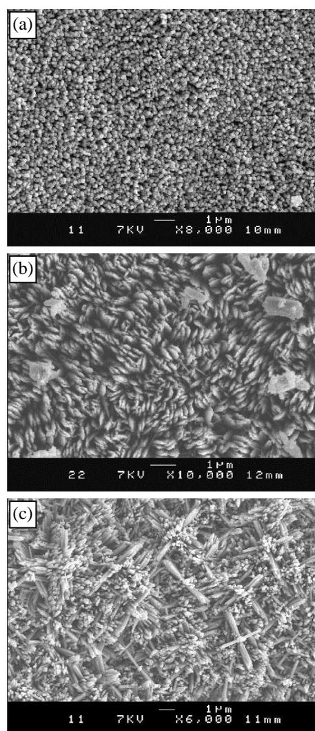
**Figure 1.** SEM micrographs showing the morphology of (a)  $\gamma$ - $\text{MnO}_2$  (49,17), (b)  $\gamma$ - $\text{MnO}_2$  (63,15) and (c)  $\alpha/\gamma$ - $\text{MnO}_2$ .
