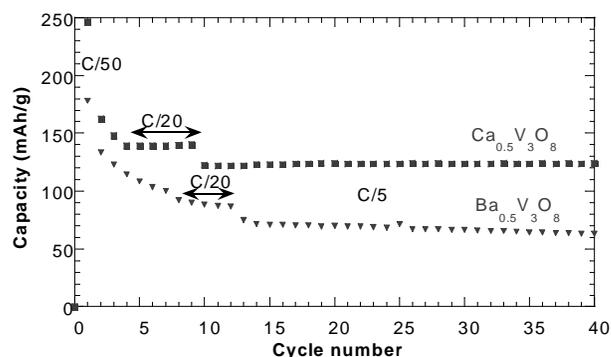
Fig.2 : Cycling behavior of two completely substituted compounds.
