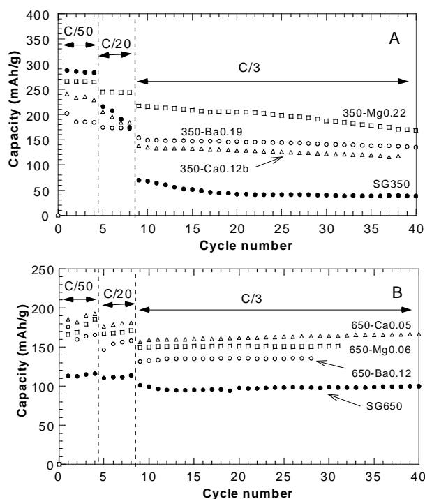
Fig.1 : Cycling behavior of several partially exchanged compounds from SG350 (A) and from SG650 (B).
