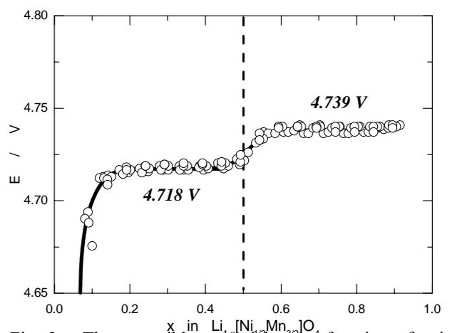
Fig. 3 The reversible potentials as a function of  $x$  in  $\text{Li}_{1-x}[\text{Ni}_{1/2}\text{Mn}_{3/2}]\text{O}_4$ .
