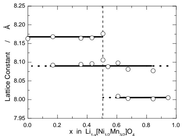
Fig. 2 Cubic lattice constant as a function of  $x$  in  $\text{Li}_{1-x}[\text{Ni}_{1/2}\text{Mn}_{3/2}]\text{O}_4$ .
