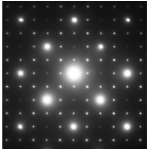
Fig. 1 Electron diffraction pattern of  $\text{Li}[\text{Ni}_{1/2}\text{Mn}_{3/2}]\text{O}_4$  prepared by a two-step solid-state reaction taken along a [100] zone axis.
