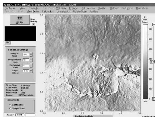
Figure 1. AFM “tapping height” image of carbon layer. This carbon layer was made by “decal process”, multi-layer hand painting using the Teflon decal, and boiled with 0.5M H<sub>2</sub>SO<sub>4</sub> and deionized water respectively. Scan box is 5×5 μm.
