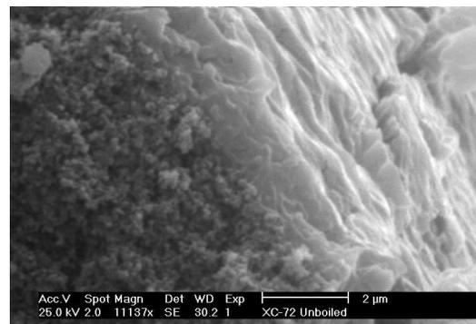
Figure 2. Scanning electron micrograph of the cross-section of the carbon layer made by multi-layer hand painting using the Teflon decal with wt. 33% Nafion®. The thickness of the white skin is approximately 0.7 μm.
