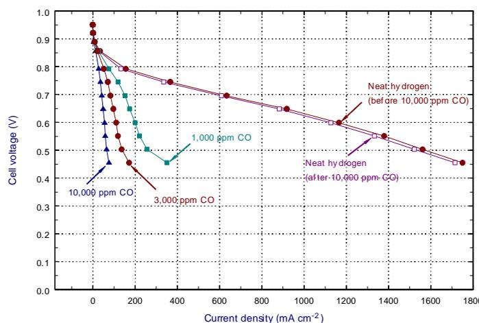
Figure 1. Effects of CO on the performance of a PEM fuel cell ( $T_{\text{cell}} = 70\text{ }^{\circ}\text{C}$ ,  $T_{\text{H}}(\text{A/C}) = 85/75\text{ }^{\circ}\text{C}$ ,  $P(\text{A/C}) = 101/101\text{ kPa}$ )
