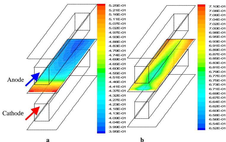
Figure 2. The distributions of local current density (Fig. 2a) and local CO coverage (Fig. 2b) on anode catalyst surface of 10-cm straight channel long PEMFC at  $V_{\text{cell}}$  of 0.4 V correspond to  $i_{\text{avg}}$  of 0.45 A/cm<sup>2</sup> for 1000 ppm concentration of CO.
