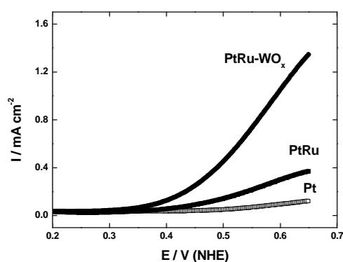
**Figure 2.** Methanol electrooxidation current density vs. potential for the PtRu- $\text{WO}_x$  nanostructured alloy electrode, PtRu, and Pt electrode.
