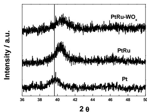
**Figure 1.** XRD patterns of Pt, PtRu, and PtRu- $\text{WO}_x$  deposited using sputtering or a multi-gun sputtering system. (The vertical solid line indicates original peak position of pure Pt in XRD pattern.)
