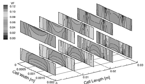
Fig. 1: Liquid water saturation inside the cathodic (lower) and anodic (upper) GDE. The channel interface area lies between between 0.5 mm and 1.5 mm.
