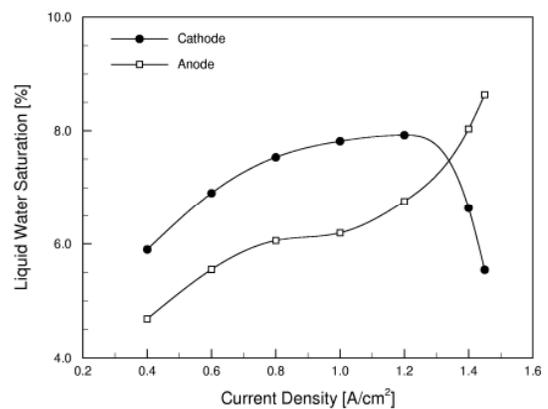
Fig. 2: Average liquid water saturation in the gas diffusion electrodes. The limiting current density is 1.5 A/cm<sup>2</sup>, and is governed by the oxygen diffusion limitation.
