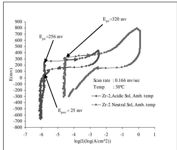
Figure 1. CPP Plot for Zr-2 in Neutral and Acidic Solutions at Ambient Temperature
