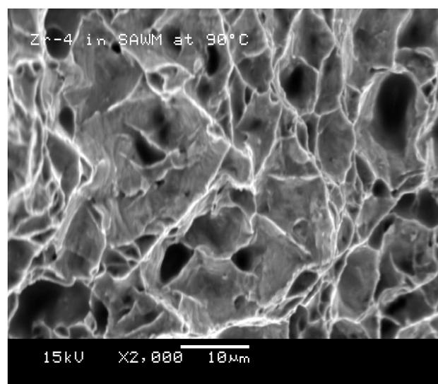
Figure 2. Micrograph of Zr-4 Fracture Surface in Acidic Solution at 90°C
