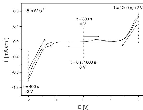
**Fig. 1** Cyclovoltammetric response of a hybrid EC device (FTO //  $WO_3$  // ICS-PPG4000 / KI /  $I_2$  / EtOH / AcOH // Pt // FTO) during *in-situ* resonance Raman measurements. The dotted lines represent the potentials at which the Raman spectra recording started.
