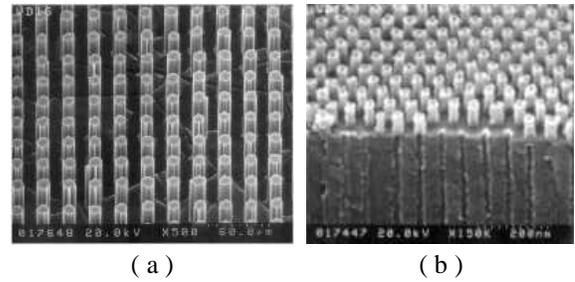
Fig.1.(a)Cross sectional view of three-dimensional nanotube blocks or towers grown selectively on 5  $\mu\text{m}$  by 5  $\mu\text{m}$  pattern. (b) Scanning electron microscope image of vertically aligned CNTs grown in the patterned nano pore.<sup>[5, 6]</sup>
