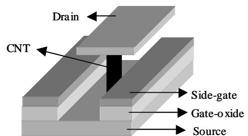
Fig.3. Schematic image of the side gate CNT-FET showing the gate, source, and drain electrodes.
