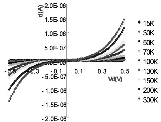
Fig.2.  $I$ - $V$  characteristic of the vertical CNT as a function of the temperature
