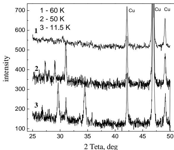
Fig 3 Low temperature XRD pattern of hydrogen-saturated C<sub>60</sub>. Note the clearly seen brightening of the lines
