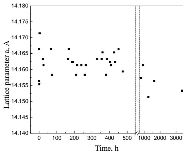
Fig 1 Dependence of the lattice parameters on the intercalation time
