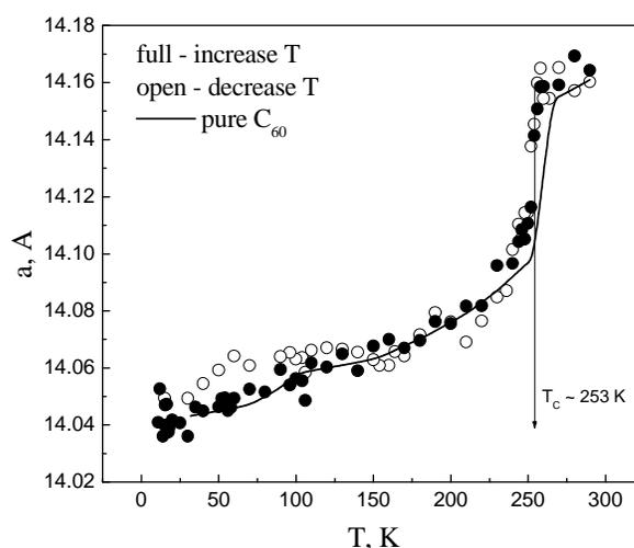
Fig 2 Temperature dependence of the lattice parameters for hydrogen saturated and pure specimens
