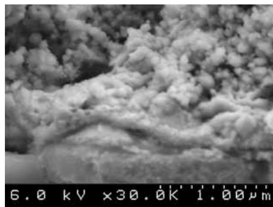
Fig. 4. A higher magnification view (of Fig. 3) reveals the porous assembly of copper nanocrystals that forms at the base of the sputter deposited coating.
