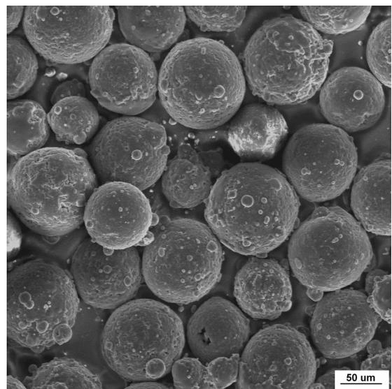
**Fig. 2 – Optical micrograph of starting Al- 21wt% Si powder fed through apparatus.**
