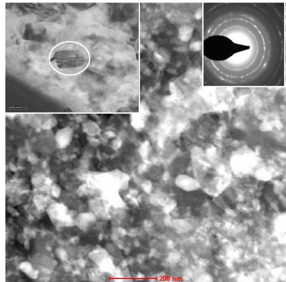
**Fig.1 – TEM micrograph of V1999-50ksi sample showing SAD 750mm image (upper right). Stacking faults (upper left). Note the fine distribution of silicon.**
