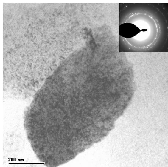
**Fig. 3 – TEM micrograph of V2000-90b sample with SAD dot and ring structure designation (upper right).**
