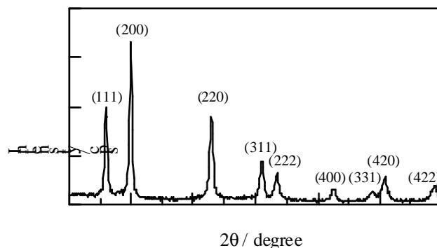
**Figure 1.** XRD patterns of the EuS nanocrystals.
