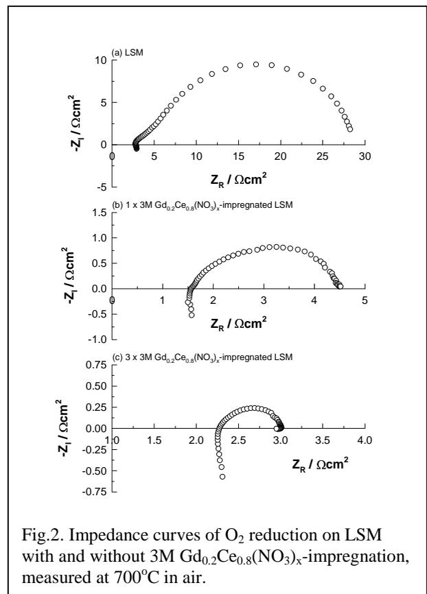
Fig.2. Impedance curves of O<sub>2</sub> reduction on LSM with and without 3M Gd<sub>0.2</sub>Ce<sub>0.8</sub>(NO<sub>3</sub>)<sub>x</sub>-impregnation, measured at 700°C in air.
