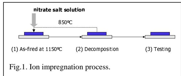
Fig.1. Ion impregnation process.
