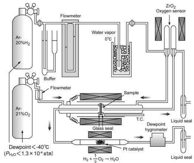
Figure 1. Experimental apparatus.
