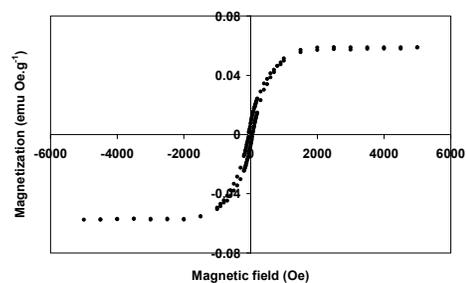
Fig. 1. Hysteresis loop at 300 K for annealed V(TCNE)<sub>x</sub> thin films
