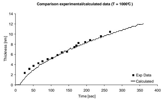
Figure 1: Comparison between calculated and experimental film thickness vs. oxidation time, at 1000°C with  $C_{O_2}^{bulk} = 3.8 \cdot 10^{-6}$  ( mol/cm<sup>3</sup>)
