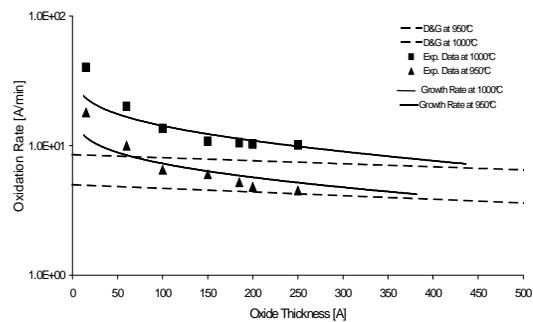
Figure 2: Comparison between the diffusion-reaction and Deal and Grove model.
