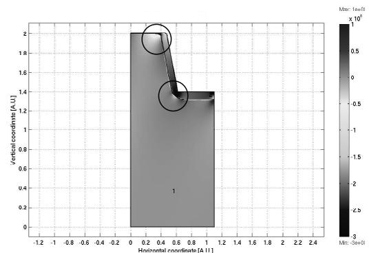
Figure 4: Lateral Stress [Pa] calculated with a 75° trench corner and 40 nm wall oxide
