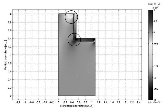
Figure 3: Lateral Stress [Pa] calculated with a 90° trench corner and 40 nm wall oxide
