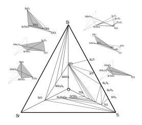
Fig. 1.The Sr-Ti-O-Si phase diagram calculated at 973.15K and 1 bar, showing some of the 9 four phase equilibria which are formed with SrTiO<sub>3</sub>. The tetrahedron presents all condensed phases which have been taken into account for the calculations.
