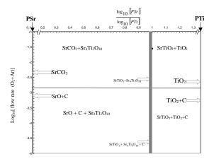
Fig 2.- Equilibrium deposited compounds as a function of precursor and Ar/O<sub>2</sub> pressure at 973.15K and 6.7 mbar
