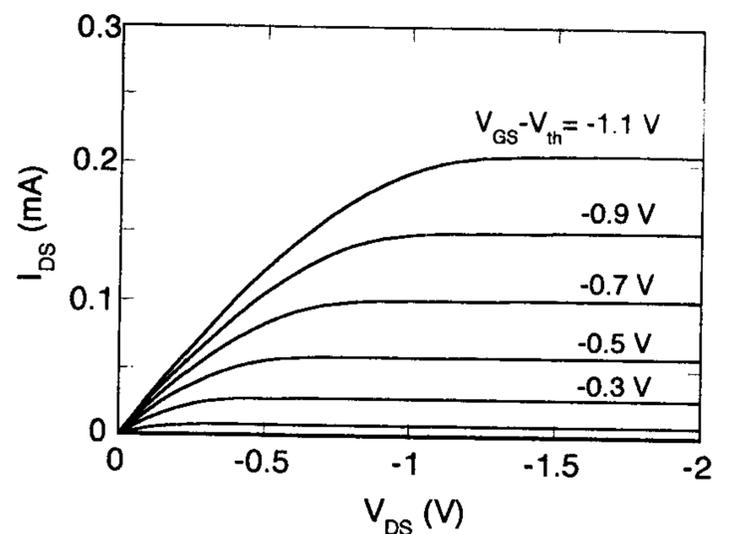
Fig. 2. I-V characteristics of the D-7 device in the saturation region
