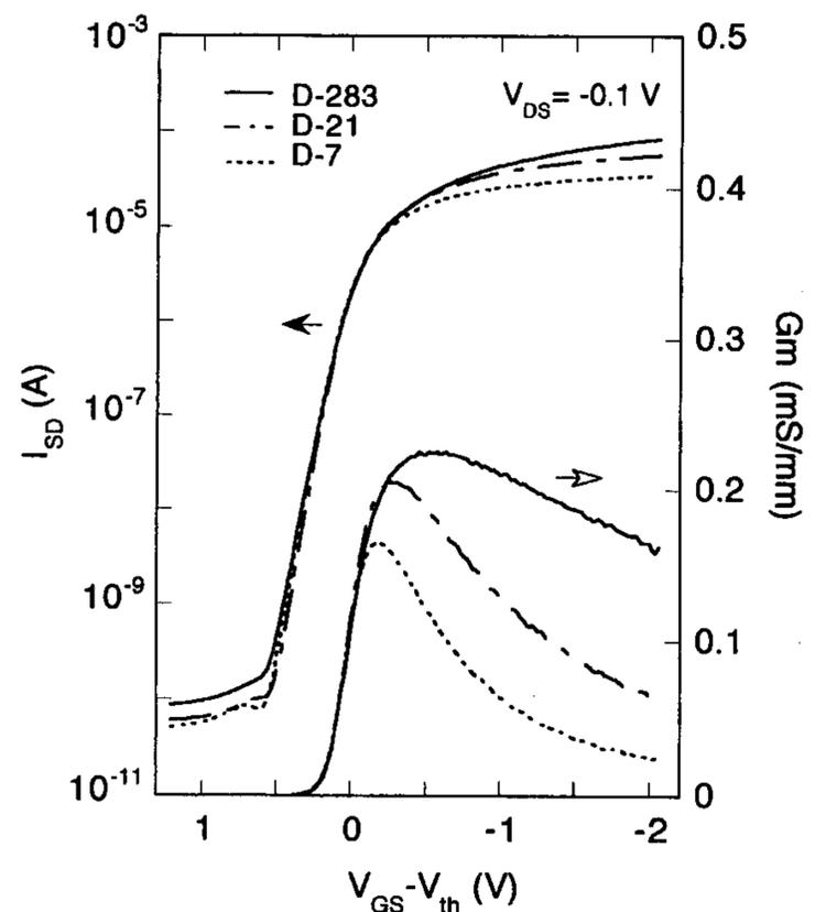
Fig. 1. Subthreshold characteristics of the devices (channel length = 10 μm, channel width = 200 μm)
