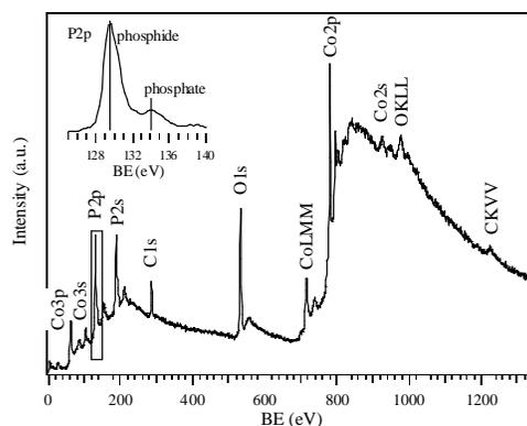
**Figure 2.** Typical surface XPS wide scan spectrum. The inset displays the P2p photopeak, evidencing the phosphide and phosphate components.
