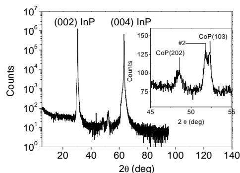
**Figure 1.** Typical X-ray diffraction spectrum (31 nm film thickness). The InP (002) and InP(004) substrate peaks are observed as well as three film peaks, shown in the inset.
