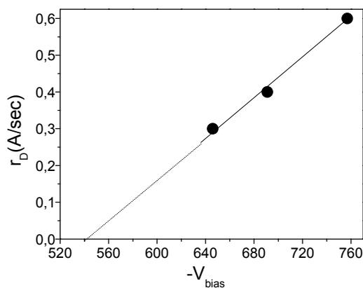
Figure 1. Dependence of Er sputtering rate on self-bias potential
