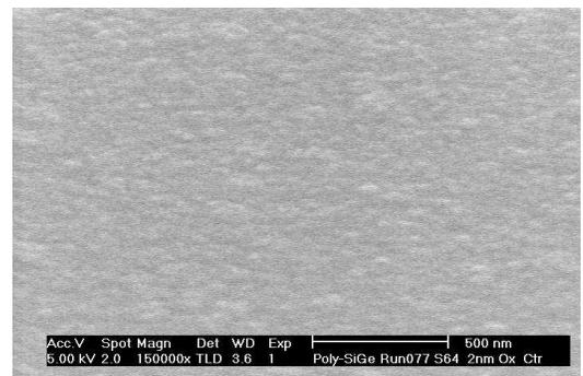
Figure 4. SEM analysis of a  $\text{Si}_{70}\text{Ge}_{30}$  film grown on a 200 mm wafer showing a void free and smooth film. The SiGe layer was deposited on a 2 nm thin furnace Gate Oxide by depositing an extremely thin (less than 1 nm) amorphous silicon seeding layer.
