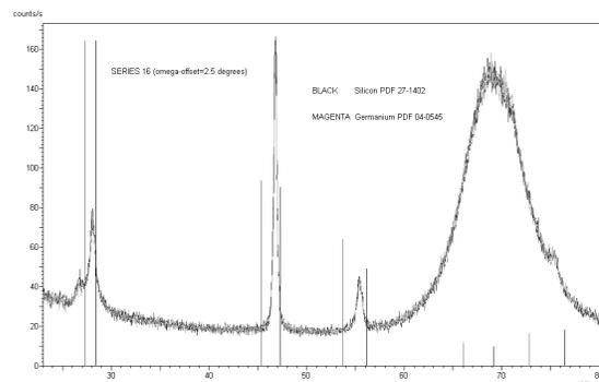
Figure 3. XRD analysis of samples taken from 3 different 300 mm test wafers distributed over the 100 Product waferload inside the vertical furnace. The three 'small' diffraction peaks arise from the polycrystalline  $\text{Si}_{70}\text{Ge}_{30}$  films with no detectable difference between the wafers.
