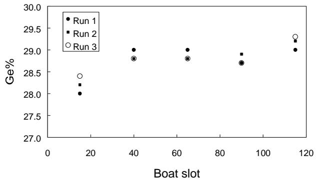
Figure 2. Ge concentration measured for three different runs. The films were deposited on 5 wafers distributed along the wafer carrier ('boat') inside the vertical furnace.
