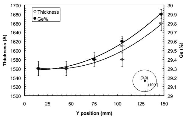
Figure 1. Within Wafer Ge concentration (right axis) and Film Thickness (left axis) as a function of position on the wafer. Film thickness and composition were determined by Rutherford Backscattering Analysis.
