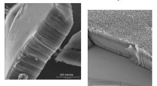
iron-rich sample (16.5 wt%) is obtained at 750  $^{\circ}$ C, and the iron-poor sample (2.6 wt%) is obtained at 850  $^{\circ}$ C which seems to be the cleanest according to SEM observations.
