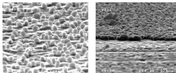
Picture 1 (a) SEM picture of the nucleation phase with Giga Copper<sup>®</sup>
