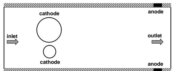
Fig. 1 The plating reactor configuration (2D cross-section)
