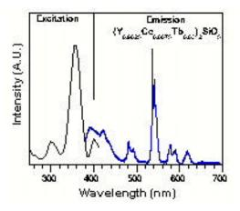
This material is based on  $Ce^{3+}$  activated  $Y_2SiO_5$ , a well-known blue emitting material. The blue emission arises from the 5*d*  ${}^{2}F_{5/2}$  and  ${}^{2}F_{7/2}$  transitions of  $Ce^{3+}$ . Co-activating with  $Tb^{3+}$ , a green emitter with the main peak at ~555 nm ( ${}^{5}D_4$   ${}^{7}F_6$ ), also produces desirable satellite peaks in the blue and red portions of the visible spectrum. The blue emission arises from the  ${}^{5}D_3$  and  ${}^{5}D_4$
