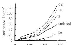
Fig.1 Luminance of cathodoluminessages for  $SrIn_2O_4$ : $Pr^{3+}$  samples at room temperature. The impurity ions were added at a nominal concentration of 5 atom.% per  $In^{3+}$  ions.
