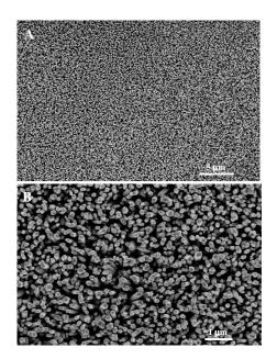
Figure. (A)-(B) top view of SEM images of ZnO nanorod arrays grown on ITO substrates pre-modified with densely and uniformly dispersed ZnO nanoparticles.
