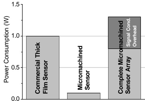
Fig.2: Comparing Power Consumptions. A full-fledged micromachined sensor array with heater driver needs about as much power as a single commercial thick film device. The additional power needed for signal conditioning electronics is also shown.
