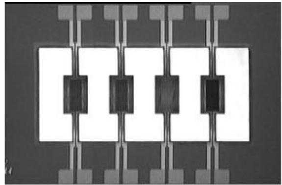
Fig.1: Top-down view of a four sensor micromachined array. The four hotplates are independently heatable. The power consumption is shown in Fig. 2
