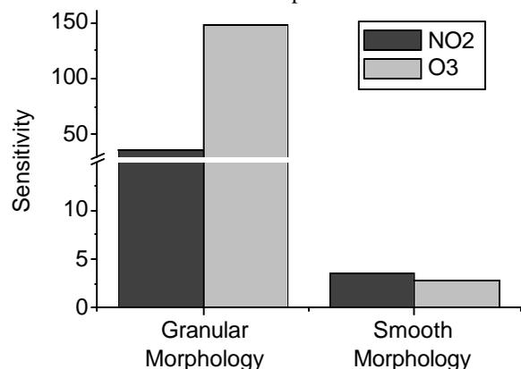
Fig.3b: Cross Sensitivity Shaping with film morphology. Tin oxide films of different morphology show different sensing patterns at the same operating temperature.
