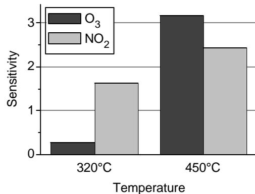
Fig.3a: Cross Sensitivity Shaping with temperature. The same kind of gas sensing material (in this case SnO<sub>2</sub>) will exhibit different cross sensitivities when operated at different temperatures.
