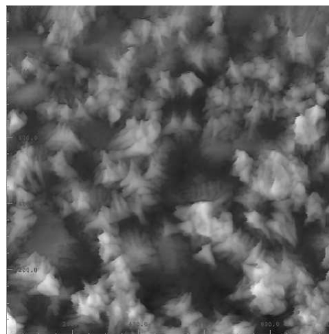
Fig. 2. In-situ 1 X 1 \mu\text{m} AFM image of approximately 50 nm of nickel deposited in the presence of saccharin. Saccharin strongly affects the morphology evolution of nickel films at higher overpotentials.
