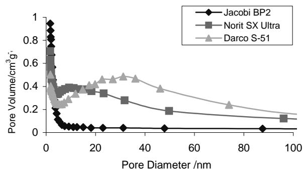
Figure 3: Pore size distribution for three ACs. BJH Adsorption.
