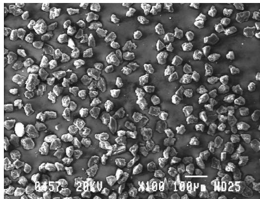
Figure 1: Micrograph of sieved particle fraction 36-38 μm.
