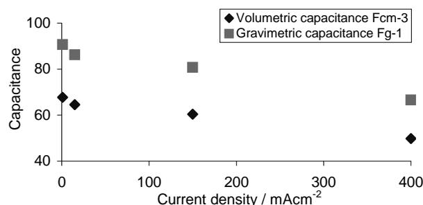
Figure 2: Volumetric capacitance of DL-electrode. AC: Jacobi Carbon BP2, particle size: <10 μm, binder : PTFE 9%.
