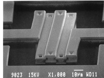
Fig. 3. SEM image of the fabricated inductor.
