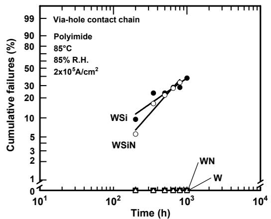
Fig. 4. Dependence of cumulative failure of via-contact chain sample on adhesive metals.
