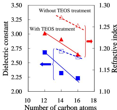
Figure 1 Dielectric constants and refractive indexes of periodic porous silica films as a function of the number of carbon atoms in alkyl chain of surfactant. Solid and open symbols represent with and without TEOS treatment, respectively.
