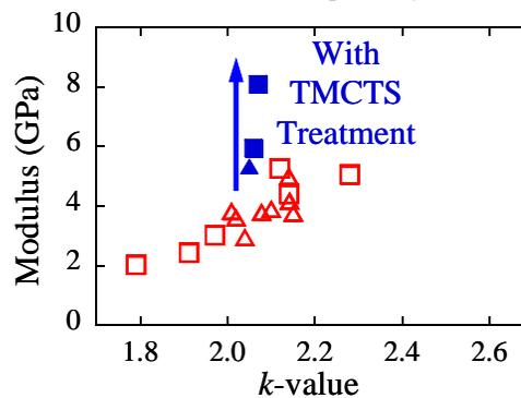
Figure 2 Elastic modulus versus  $k$ -value for disordered porous silica low- $k$  with or without TMCTS treatment.
