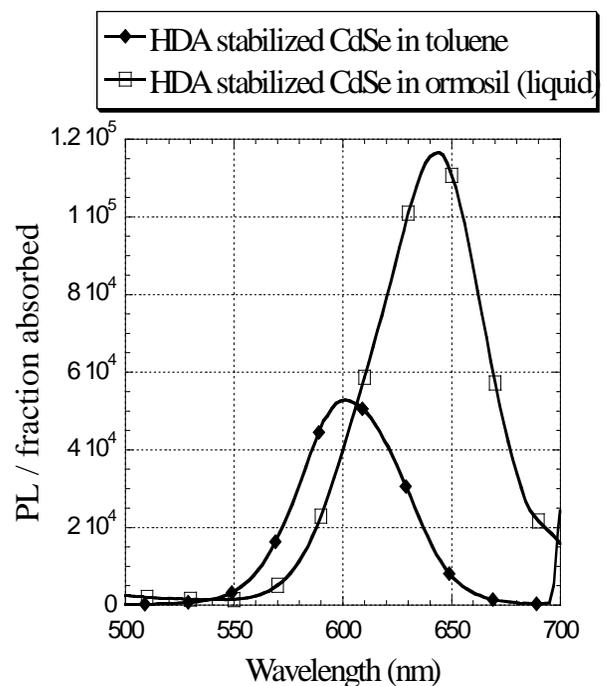
Figure 1. Enhancement of luminescence of HDA (hexadecylamine) stabilized CdSe nanoparticles via dispersion in ormosil.
