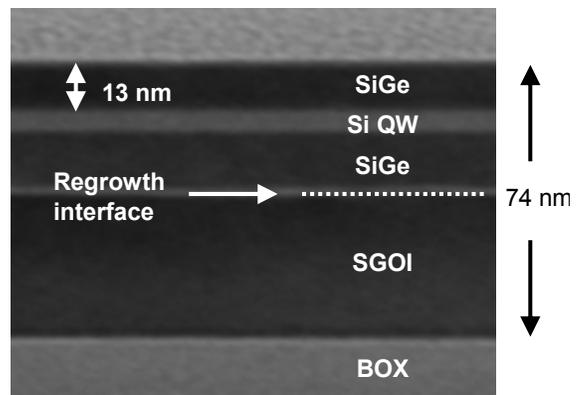
Fig. 3. Cross-sectional TEM micrograph of a Si/Si<sub>0.7</sub>Ge<sub>0.3</sub> layer structure grown on a thin SGOI substrate. The initial and final SGOI thicknesses are 38 nm and 74 nm, respectively.
