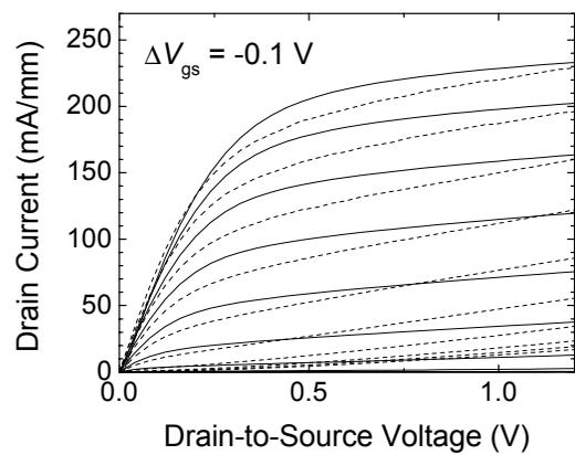
Fig. 2. Output characteristics for Si/Si<sub>0.7</sub>Ge<sub>0.3</sub> n-MODFETs with (lines) and without (dashes) p-well doping. Both devices have  $L_g = 150$  nm and  $L_{ds} = 300$  nm. The MODFETs with p-well doping have 2x lower output conductance, and improved pinch off.
