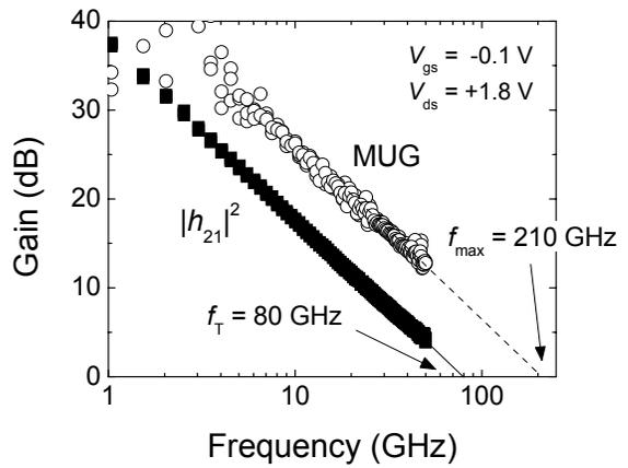
Fig. 1. Plot of  $|h_{21}|^2$  and MUG vs. frequency for a Si/Si<sub>0.7</sub>Ge<sub>0.3</sub> n-MODFET with  $f_T = 80$  GHz and  $f_{max} = 210$  GHz. The device has  $L_g = 80$  nm, and  $L_{ds} = 300$  nm and a total gate width of 20  $\mu$ m.
