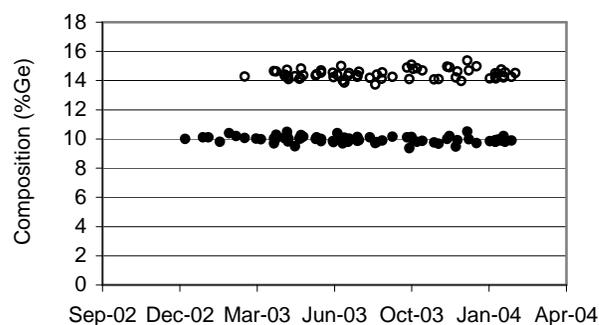
Fig. 3. Long-term reproducibility of Ge composition. (Open circles, 14.45% SiGe box control sample; filled circles, 0-10% SiGe grade control sample – maximum value plotted)
