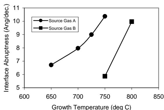
Fig. 2. Interface Abruptness versus growth temperature and source gas (A=SiH<sub>4</sub>, B=SiH<sub>2</sub>Cl<sub>2</sub>)
