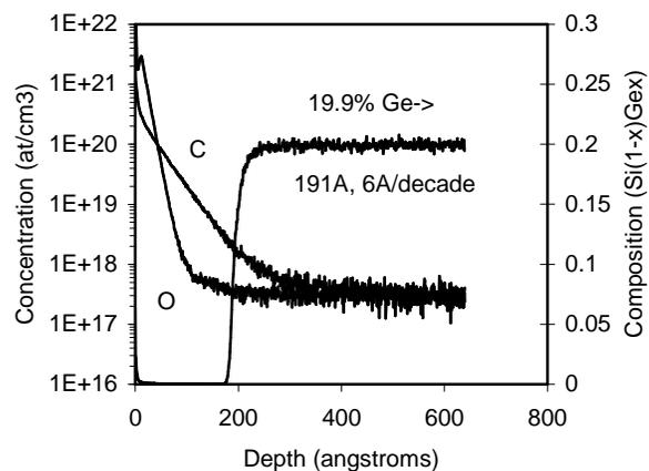
Fig. 1. ULE SIMS Profile, strained Si on SiGe buffer layer. A single profile can demonstrate the thickness of the strained Si cap, Ge composition, interface abruptness and atmospheric contamination with high sensitivity.
