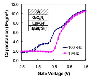
**Figure 3.** Bi-directional CV characteristics of epi-Ge MOS capacitors with GeO<sub>x</sub>N<sub>y</sub> gate dielectric and W gate electrode: 100 kHz and 1 MHz.
