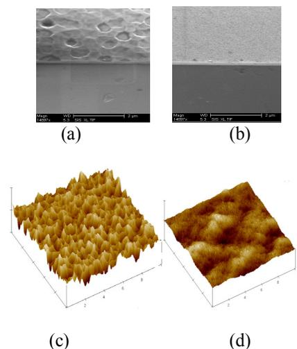
**Figure 1.** Cross section HR-SEM image of (a) No anneal (b) 825°C H<sub>2</sub> anneal; Surface AFM image of epi-Ge layer: (10μm X 10μm) (c): No anneal, (d) 825°C H<sub>2</sub> anneal.
