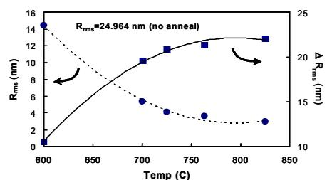
**Figure 2 (left axis data)** RMS of epi-Ge layers as a function of hydrogen annealing temp for 1 hr measured by AFM. (10μm X 10μm) (**right axis solid**) change in RMS (RMS (No anneal) – RMS (Anneal), vs TEMP (RMS of the non-annealed sample if 24.94 (nm) (fitted)
