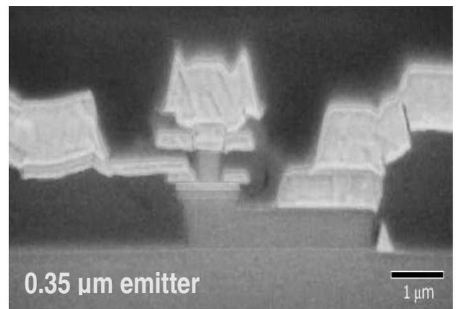
FIG.2. SEM Cross-section of a 0.35 μm device
