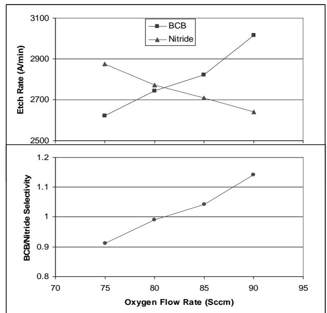
FIG. 3. BCB And Nitride Etch Rates And Selectivity vs O<sub>2</sub> Flow Rate. Power=150w; Pressure=300mtorr; SF<sub>6</sub>=15sccm; Temperature=25C
