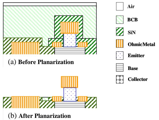
FIG.1. BCB/SiN Planarization Process Flow
