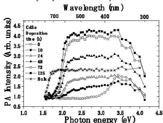
Fig. 2. PA spectra of TiO<sub>2</sub> electrodes adsorbed with CdSe QDs for different adsorption time.
