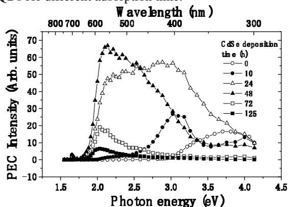
Fig. 3. PEC spectra of TiO<sub>2</sub> electrodes adsorbed with CdSe QDs for different adsorption time.
