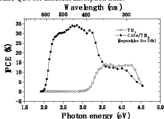
Fig. 4. IPCE spectra of TiO<sub>2</sub> electrode (○) and that with CdSe QDs adsorption (●) for 24 hours.
