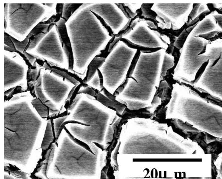
Fig. 1. SEM micrograph image of the TiO<sub>2</sub> electrode made from hydrolysis and oxidation processes of TiCl<sub>4</sub>.
