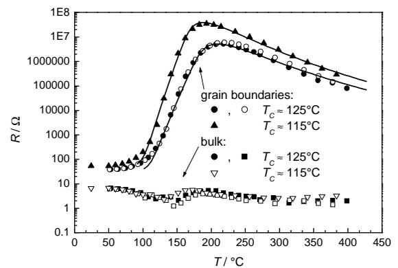
Fig. 1 Temperature dependence of bulk and grain boundary resistances of n-conducting BaTiO<sub>3</sub> ceramics with different Curie points ( $T_C$ ). Sample dimensions: 2.2 mm thickness, 8.0 mm diameter. The solid lines have been calculated according to the Heywang model (Schottky-barrier-model).
