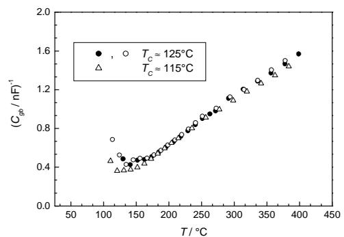
Fig. 2 Reciprocal grain boundary capacitance of n-conducting BaTiO<sub>3</sub> ceramics with different Curie points ( $T_C$ ) plotted versus temperature. Sample dimensions: 2.2 mm thickness, 8.0 mm diameter.
