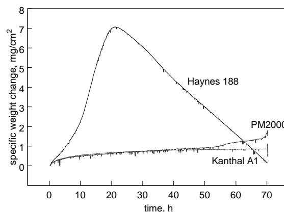
Figure 2. Specific weight change for coiled wires exposed at 1204°C, in 50% H<sub>2</sub>O/50% O<sub>2</sub> flowing at 4.4 cm/s.
