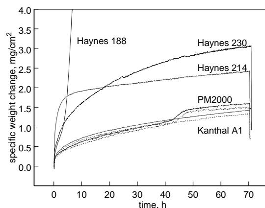
Figure 1. Specific weight change for coiled wires exposed at 1204°C, in dry O<sub>2</sub> flowing at 0.4 cm/s.
