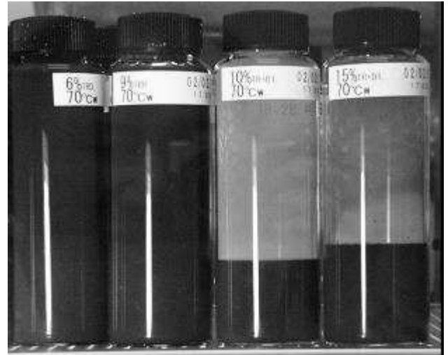
Fig.1 Photo image after heat treatment of various concentration of Triton X-100 at 70°C. After 15 hr.
