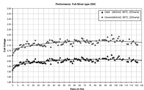
The most important achievement of this type of configuration is the stability of the system also during uncontrolled shut-down, providing that the cell is protected with a polarization rectifier. Some results of the systematic approach used to understand the behavior of the system during various possible conditions occurring during shut down will be discussed, including some interpretation of the operating data, mainly during the first days of cell operation.
