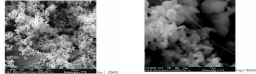
The catalyst is incorporated into a gas diffusion electrode structure, that contains a Ag net used to support the catalyst mass and distribute the current. The construction of the electrode is simple, and no structural differences exist at the moment between the gas and the liquid side.
