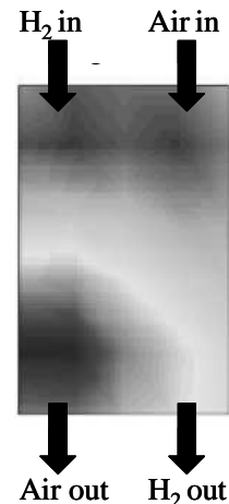
Fig. 1: Standard technique Influence of the increase in air stoichiometry ratio from \lambda_{Air}=2 to \lambda_{Air}=4 on the current density distribution (blue : decreased current density at the air inlet red: increased current density at the air outlet) (operating conditions: 2 bar, 70°C active area: 244 cm 2 )
