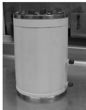
Figure 1. Inert chambers for accelerated life testing and isolated component leachate analysis.
