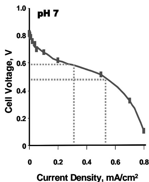
Fig. 2: Polarization curves of the biofuel cell gas-diffusion air cathode with BOD as oxygen reduction electrocatalyst and glucose oxidation anode based on mediated nickelocene/glucose oxidase electrode.
