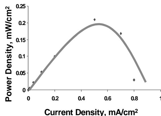
Fig. 3: Dependence of the power derived from the glucose-air biofuel cell on the current density.
