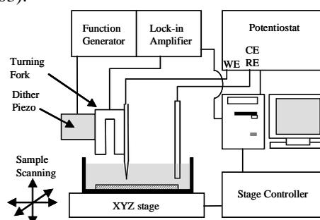
Fig.1 Schematic diagram of the SECM with shear force feedback.
