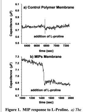
control membrane shows no response to L-Frome. a) The control membrane shows no response to the addition of  $6.5 \times 10^{-6}$  M L-Proline, The MIP membrane responds to addition of  $6.5 \times 10^{-6}$  M L-Proline, while the control membrane does not.
